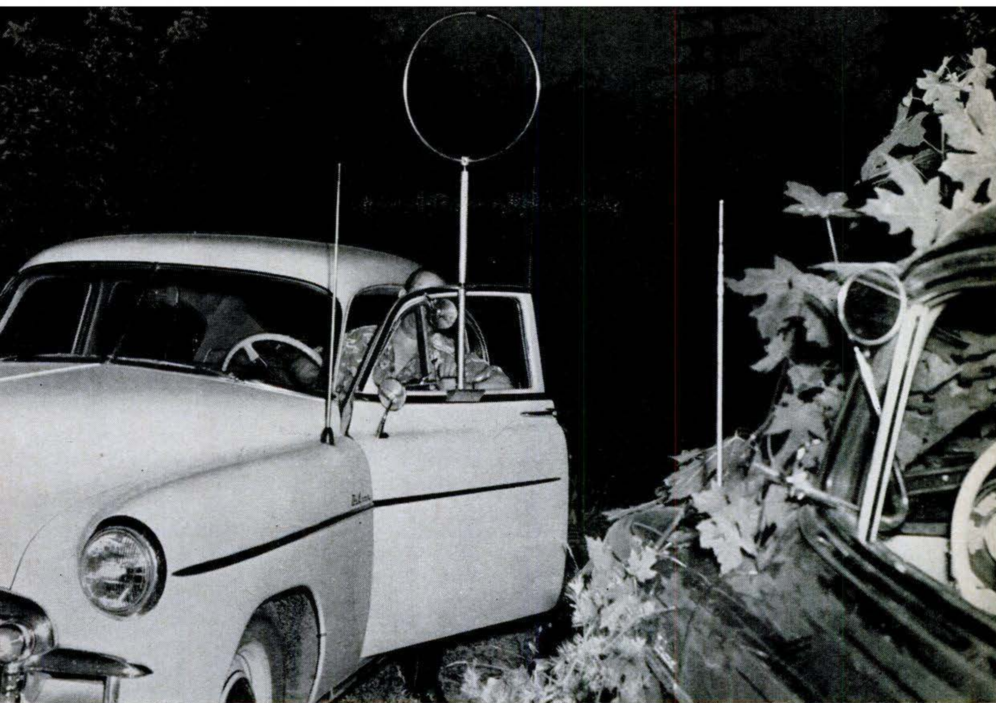
Transmitter in hidden car (right) was tracked down with the help of revolving loop antenna.
